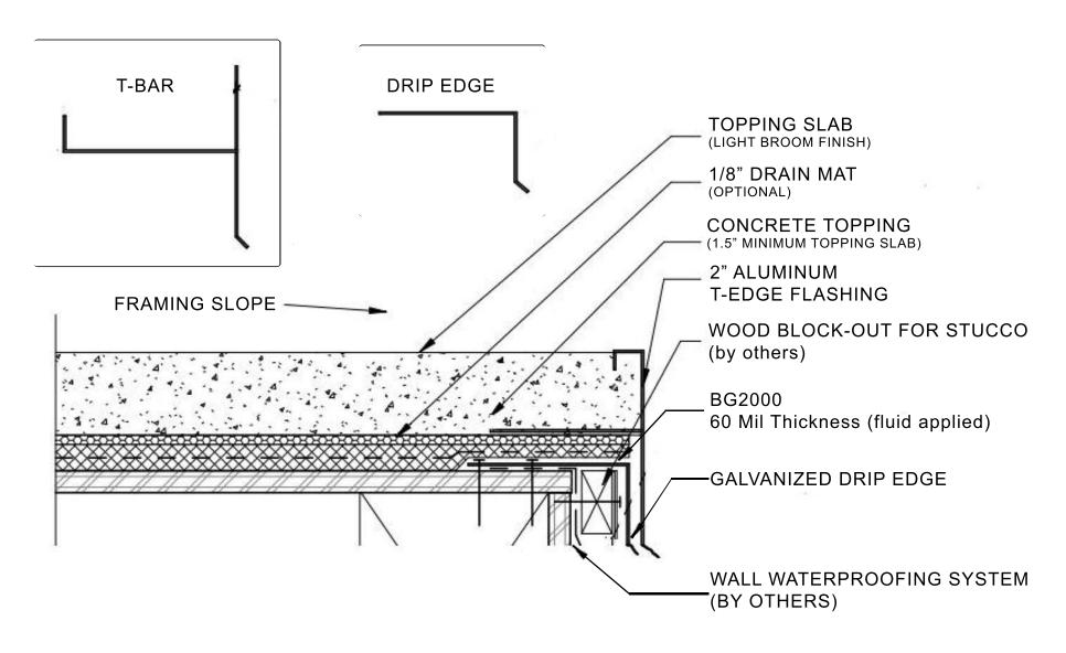
Pre-sloped plywood or OSB Substrate 2% maximum
